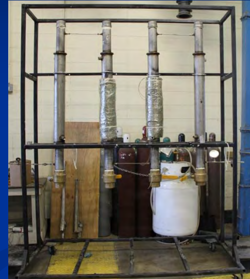
Pilot-scale syngas cleaning system
